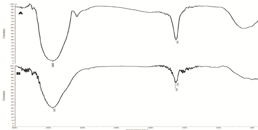
**Fig. 2:** FT-IR confirmed the coupling between carboxylated SPIONs and amino group in ASO. (A) SPIONs (B) ASPIONs-ASO
