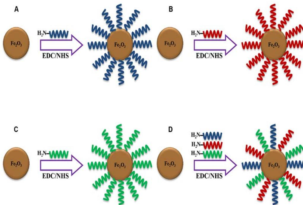
**Fig. 1:** Schematic representation for SPIONs-ASO conjugates. A, S-M1; B, S-M2; C, S-M3; S-M4
